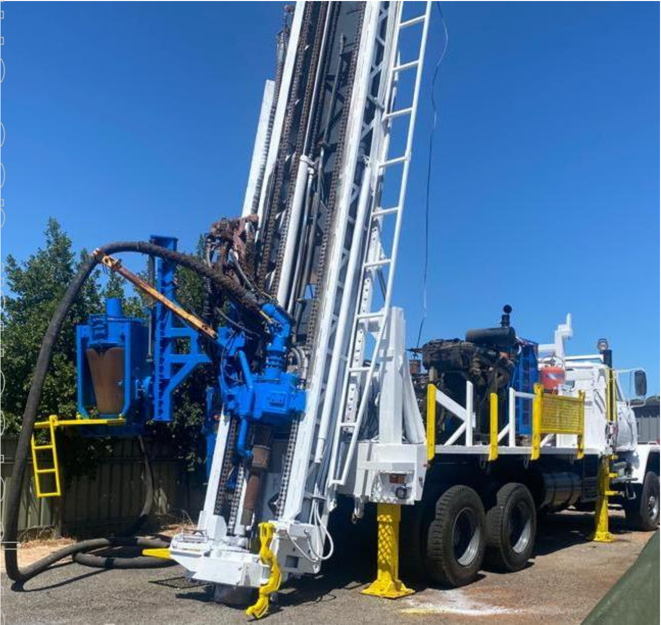
Image 2: Company's Schram 450 RC drill rig awaiting deployment.
