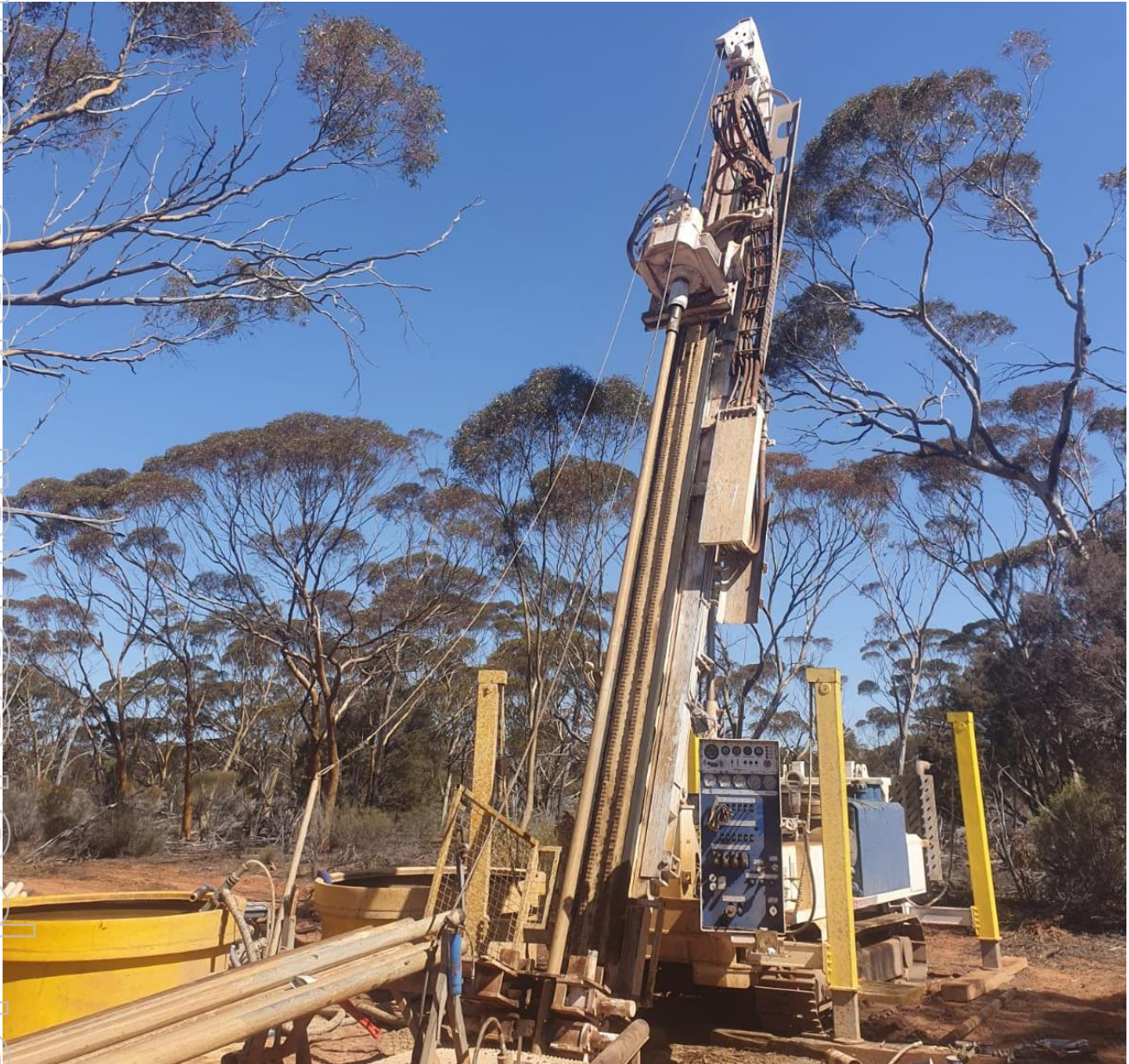
Image 1: Company's Desco SP7000S diamond drill rig over first Grindall diamond hole.
