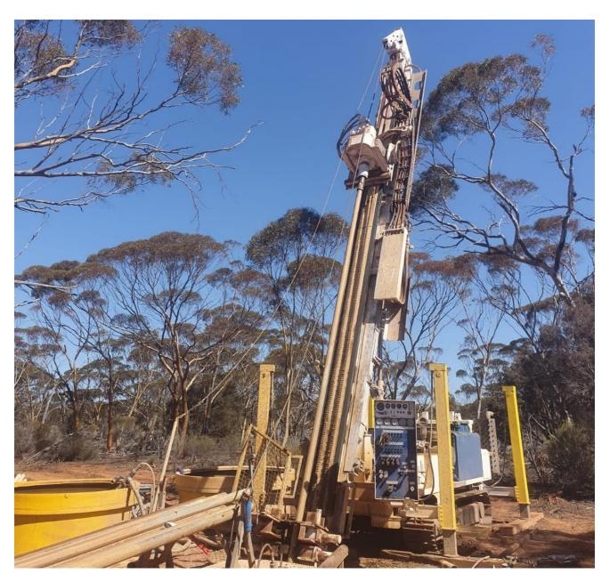
Image 1: Company's Desco SP7000S (WOC) diamond drill rig over first Grindall diamond hole.
