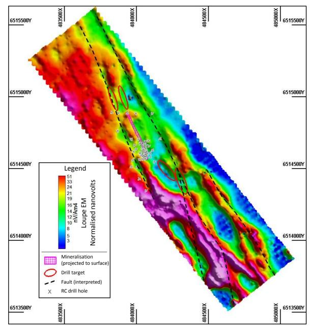
Image 2: Socrates Loupe electromagnetic survey showing existing RC drill holes, interpreted faults and targets for drilling in 2021.
