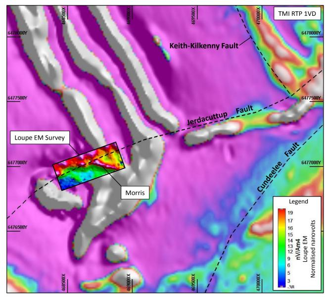
Image 3: Loupe electromagnetic survey showing the conductor identified at the Morris Prospect as well as the regional total magnetic intensity, reduced to pole, first vertical derivative.
